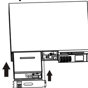
After replacing the batteries, put the battery box back to original location and screw it tightly.
