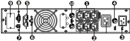
1. Programmable outlets: connect to non-critical loads.
