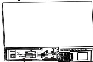
Disconnect battery wires.
