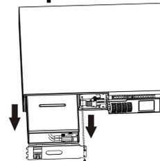
Pull out the battery box by removing two screws on the front panel.
