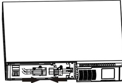
Connect the AC input and re-connect battery wires.
